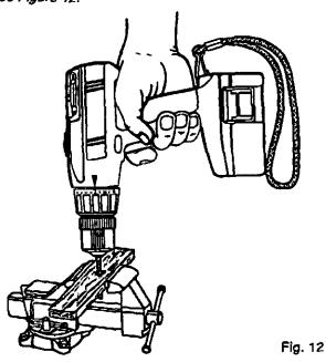
When drilling hard smooth surfaces use a center punch to mark desired hole location. This will prevent the drill bit from slipping off center as the hole is started. However, the low speed feature allows starting holes without center punching if desired. To accomplish this, simply operate your drill at a low speed until the hole is started.
